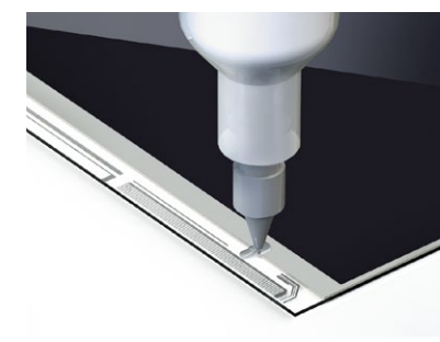
Conductive Ag paste dispensing on touch panels
