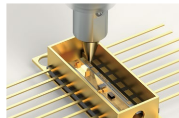
Dispensing Ag Paste on optical communication module
